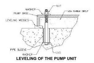
Lower the pump onto the foundation, positioning the pump so the anchor bolts are aligned in the middle of the holes.
